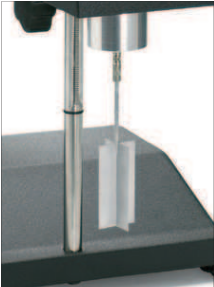
The instrument shown is a DV-III Ultra. These spindles also work well with other Brookfield Viscometers.
