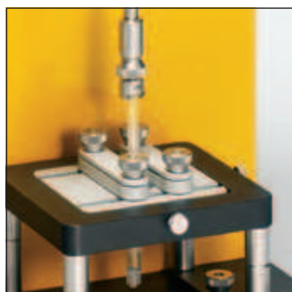
CT3 Texture Analyzer (p58) with Syringe Test Fixture
